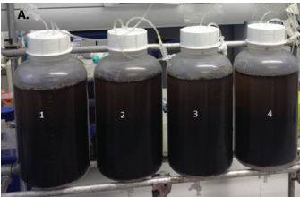
Figure 9: Investigation of effect of lignin-degrading bacteria on the anaerobic digestion of commercially available compost.
