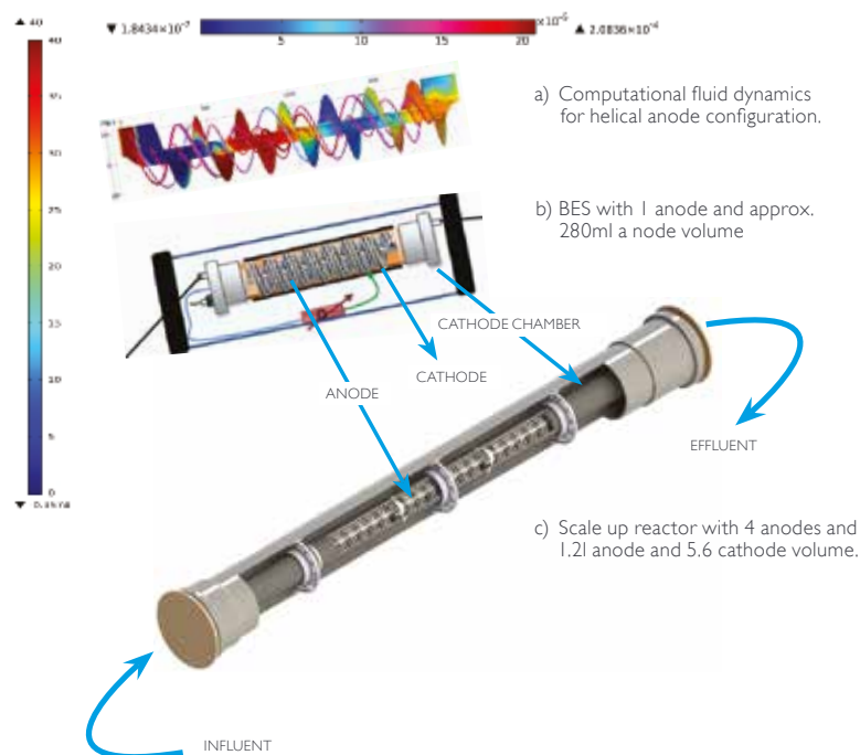
Figure 14: Surface plot showing acetate concentration (mol min -1 ) on helical side wall and streamlines showing fluid flow (b) One reactor module containing 1 anode and 1 cathode which can be scale up to (c) multiple anode and cathode assembly in one reactor system
