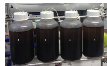
Figure 9: Investigation of effect of lignin-degrading bacteria on the anaerobic digestion of commercially available compost.
